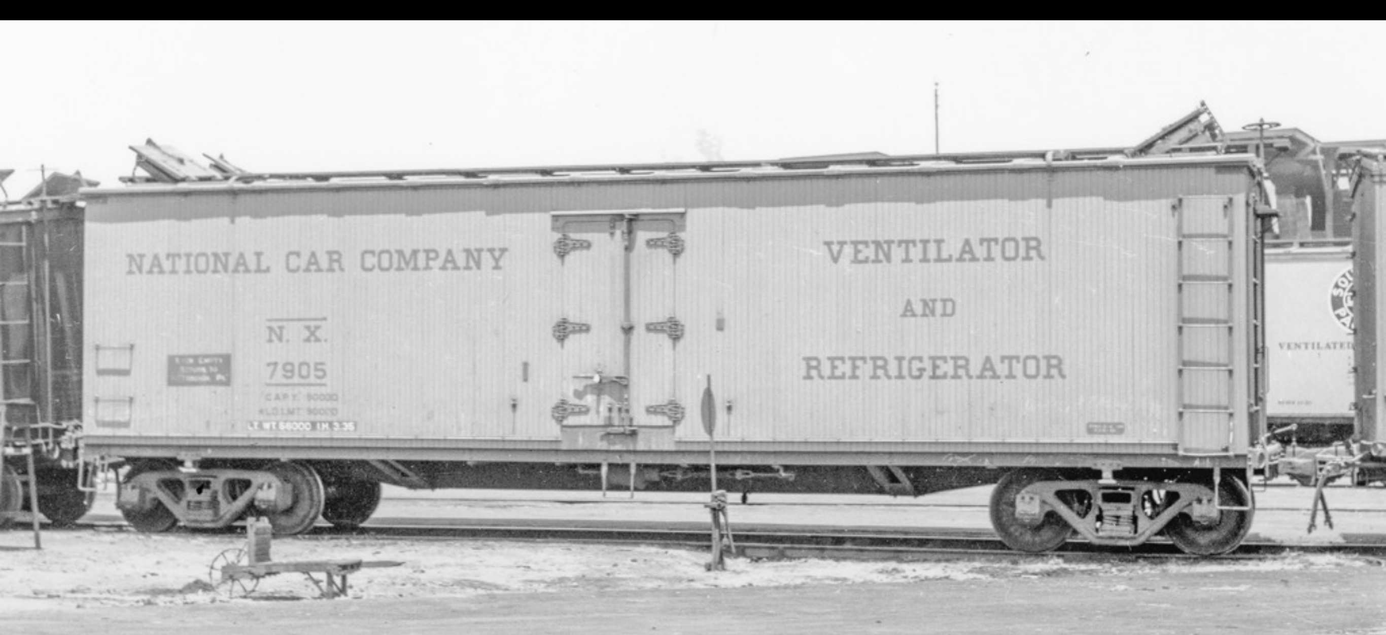
Fruit Growers Express/National Car R7 underframe Refrigerator Car
