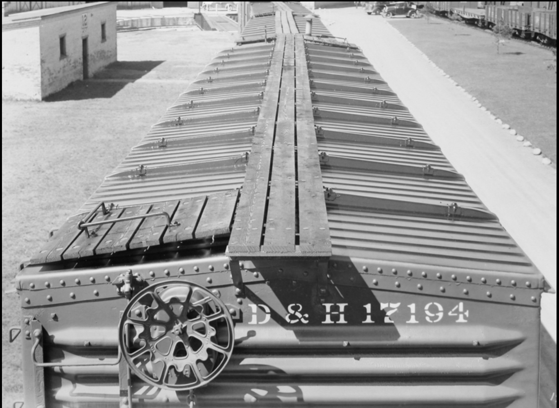
Delaware & Hudson USRA 50-ton Box Car with Viking corrugated steel roof
