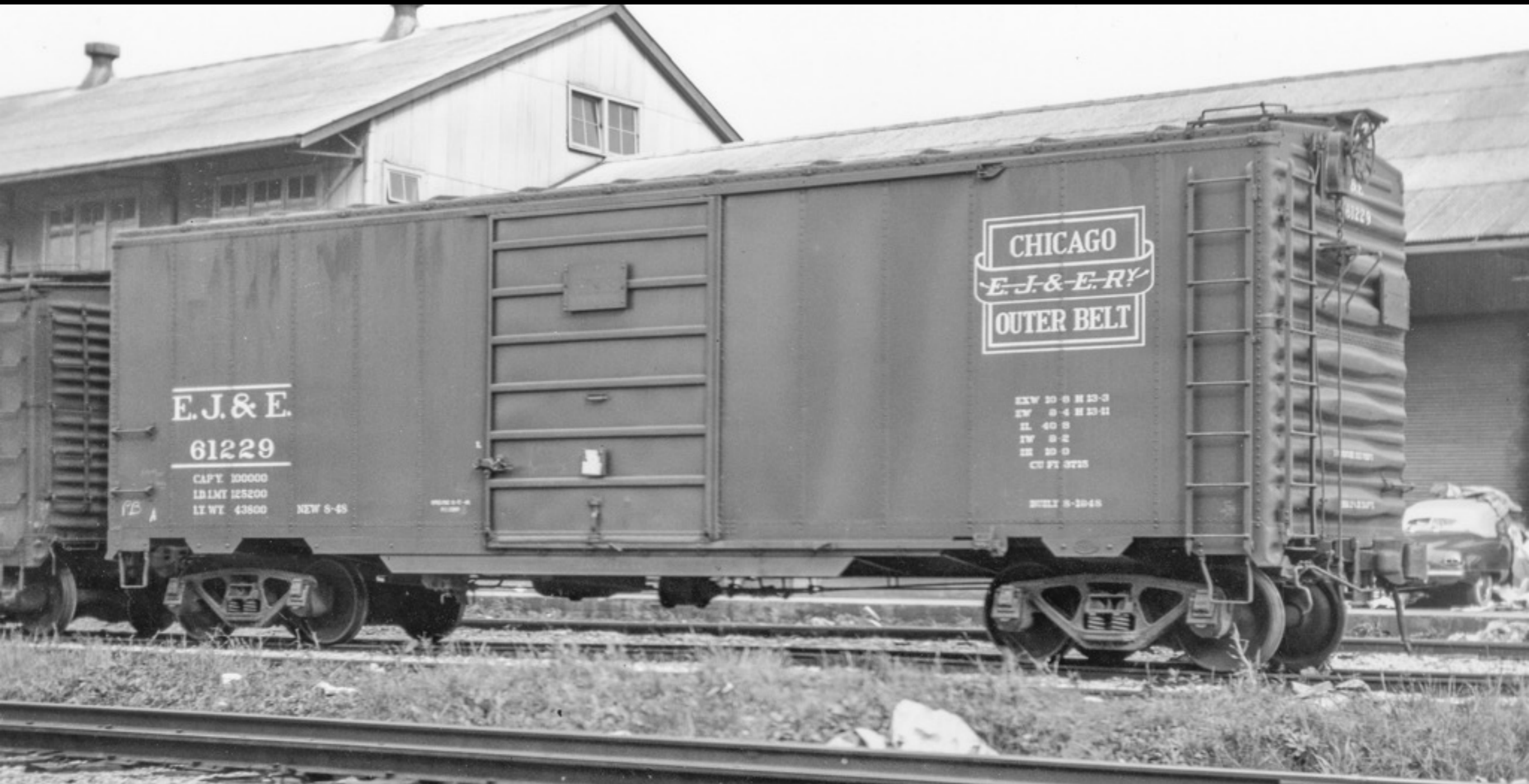
Elgin, Joliet & Eastern 10'0" inside height 12-panel postwar AAR box car
