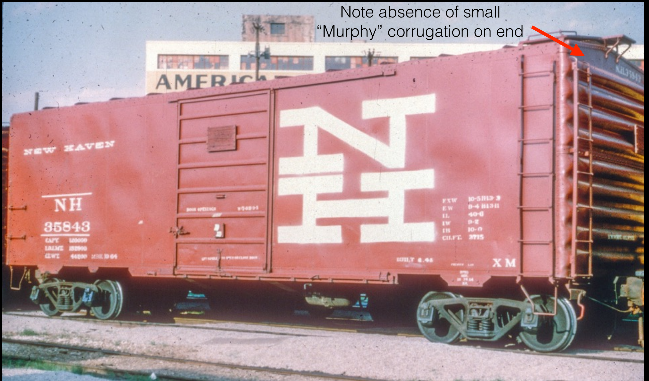
New Haven 10'0" inside height PS-1 box car
