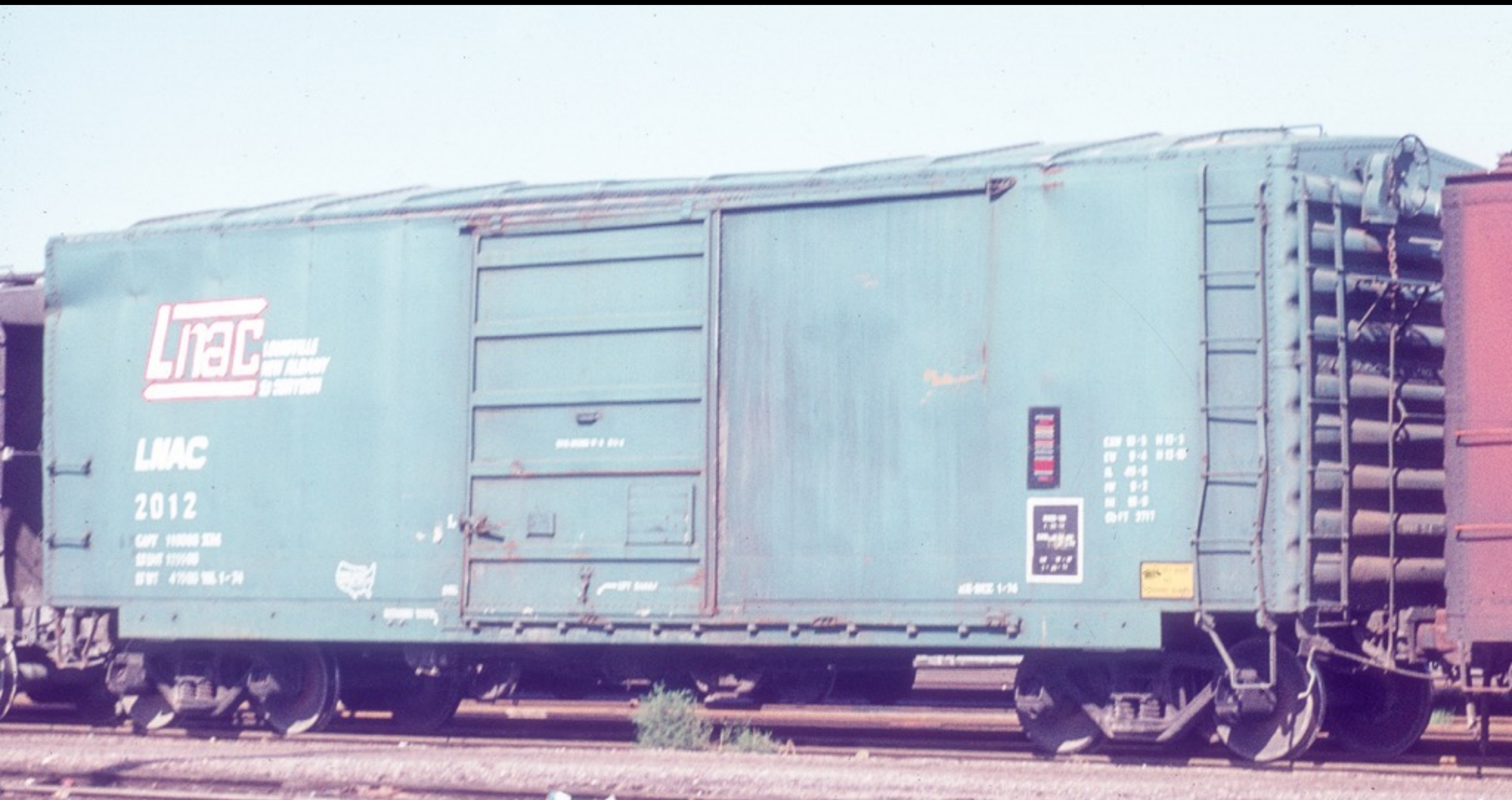
Louisville, New Albany & Corydon ex-New Haven 10'0" inside height PS-1 box car
