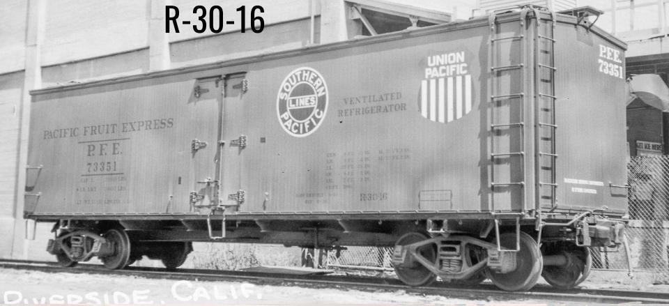
PFE 73351 was a -16 repainted in 1947 in the '1946' P&L scheme. It still had its KC schedule brakes. It used a 30-ton built-up underframe
