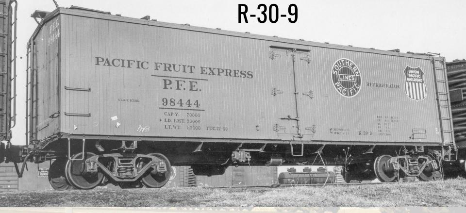
This photo of R-30-9 98444 affords a great view of the 30-ton built-up underframe. It was equipped with Equipco integral hatch covers
