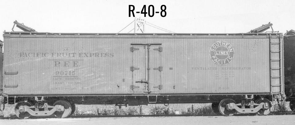
PFE 90715 was an R-40-8 built\* in October, 1932. It is notable for the Simplex trucks and enameled sheet metal medallions screwed to the car side, introduced ca. 1928 and phased out ca. early 1937 \*the R-40-8 rebuilds were stenciled "BUILT" as opposed to the rebuilt R-30-11-8 cars that were stenciled "REBLT." likely because the 30-ton cars retained the original underframes while the 40-ton cars retained little save hardware from the original cars
