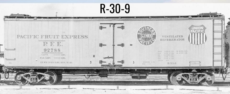
PFE R-30-9 shown after repainting at Roseville in October, 1946 in the then-current P&L scheme. Note that it has been upgraded with AB brakes and retains its wood hatch platforms
