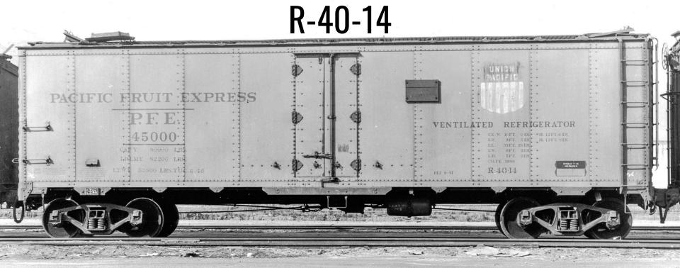
R-40-14 PFE 45000 was repainted at Tucson in 1945. Note the placard board to the right of the door. Placard and route card boards were not used on the R-40-10 class at building
