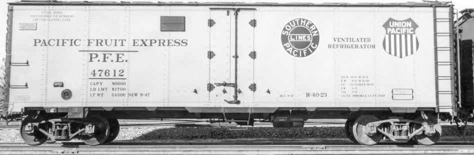
R-40-23 PFE 47612 shown soon after building. Note the locations of the placard board and route card board (at the left body bolster) as well as the ASF A-3 Ride Control trucks. These cars were the first built new to employ the 1946 P&L scheme with both medallions on each side of the car body
