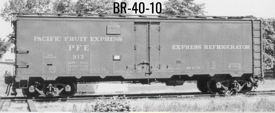
In 1952, Railway Express Agency experienced a shortage of express refrigerator cars. To help alleviate the strain, PFE modified 50 R-40-10 reefers for express service. Changes included addition of steam and signal lines, steel running boards, electric fans, and Chrysler FR-5-D or Symington-Gould Type XL express trucks
