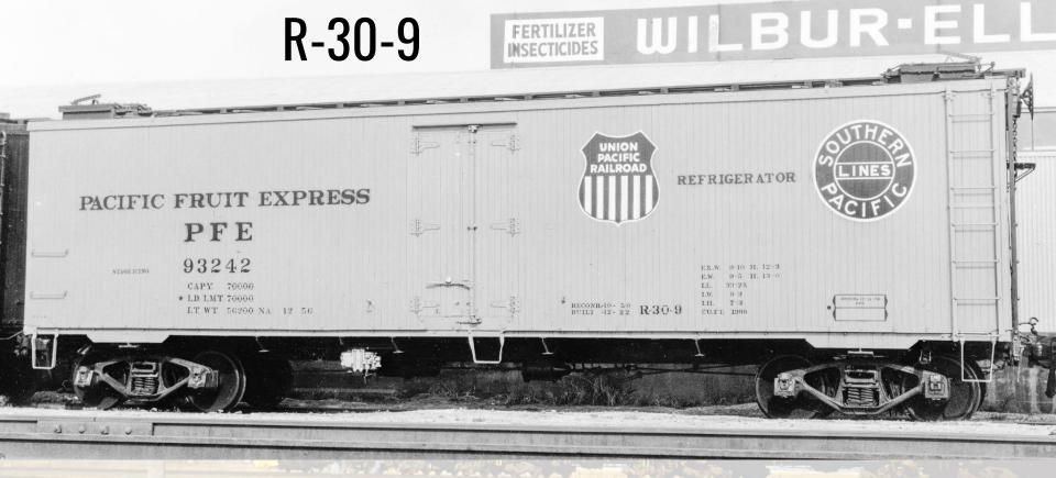
This -9 illustrates the P&L scheme introduced in 1954. Also of note are the fairly long structural enhancements at the body bolsters
