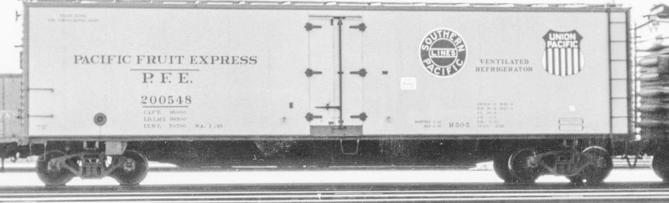
Rebuilt from R-50-1 class at Nampa between 1945-1947, car nos. 200301-200375 (tongue and groove and circa 1945 lettering) and 200379-200587 (plywood and circa 1946 lettering) with air circulating fans and seven-inch insulation for frozen food service. Note the reversed red and white in the UP medallion
