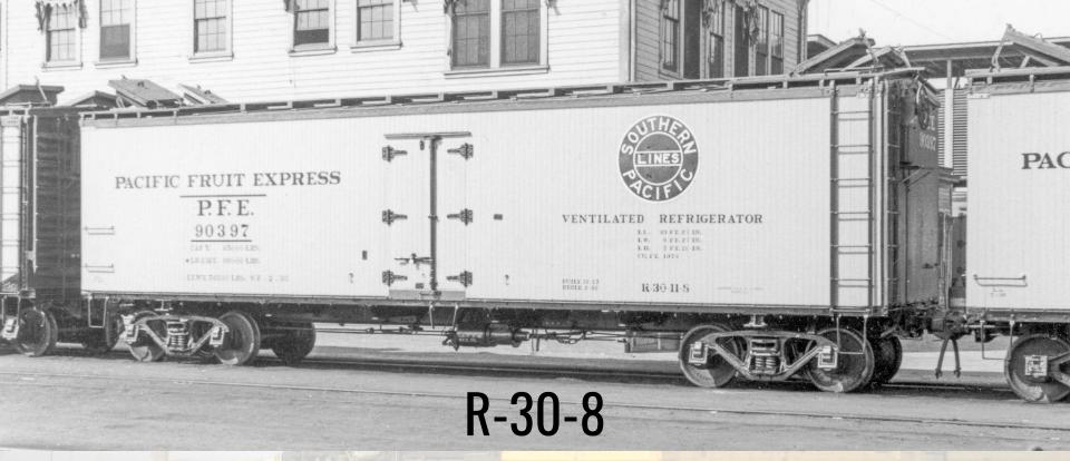
PFE 90397 differs from the other -8 rebuilds shown in that it was rebuilt from an R-30-11, retaining the original 30-ton Bettendorf underframe
