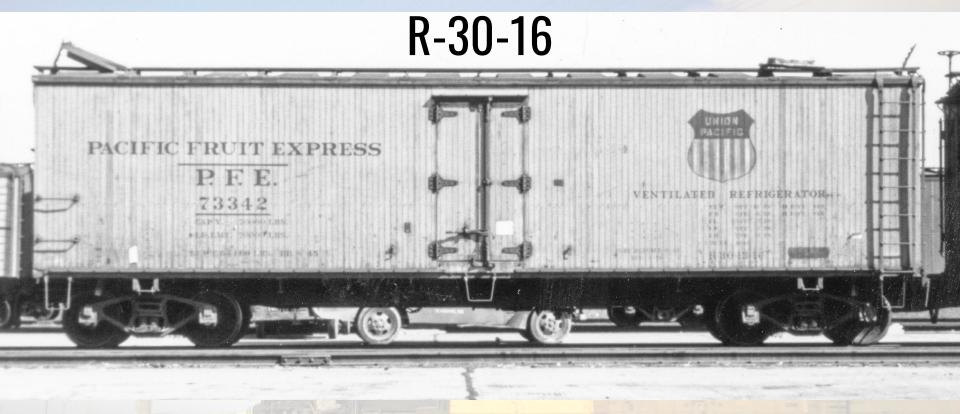
PFE 73342 was a -16 that was repainted shortly after its rebuilding, although the reason is not evident. It retained its KC schedule brakes
