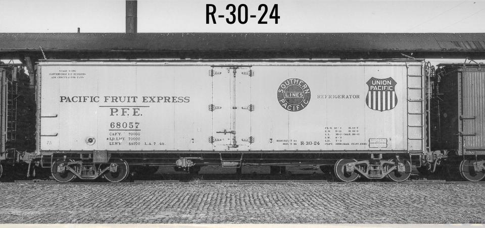
The full-height door openings and new trucks (ASF A-3 Ride Control) are evident in this image, along with the plywood sheathing
