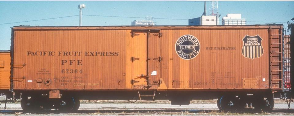
This early 60s photo shows a car with replacement tongue and groove sheathing. Of interest are the "clean" replacement sheathing boards Collection of Ted Culotta
