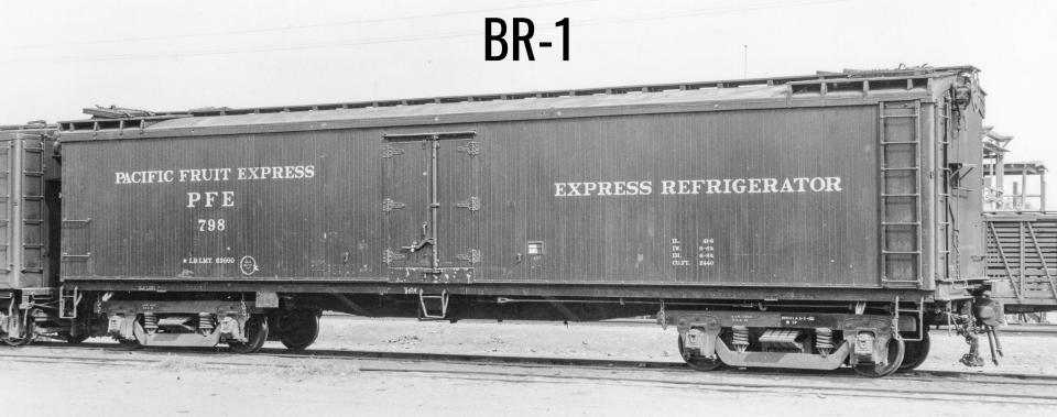
Built 1923-1924 by AC&F and General American for express service in passenger consists, car nos. 500-799. In 1952, 55 cars received heavy repairs and in 1954, 83 cars were rebuilt at Nampa, including steel superstructures, increased insulation, Preco electric fans, and steel channel side sills
