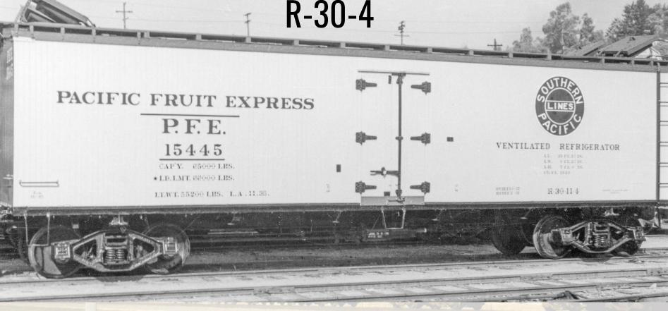
PFE 15445 was rebuilt in 1931 from an R-30-11 and designated in class R-30-11-4, subsequently shortened to R-30-4 with the updating of painting and lettering (P&L) standards of 1944
