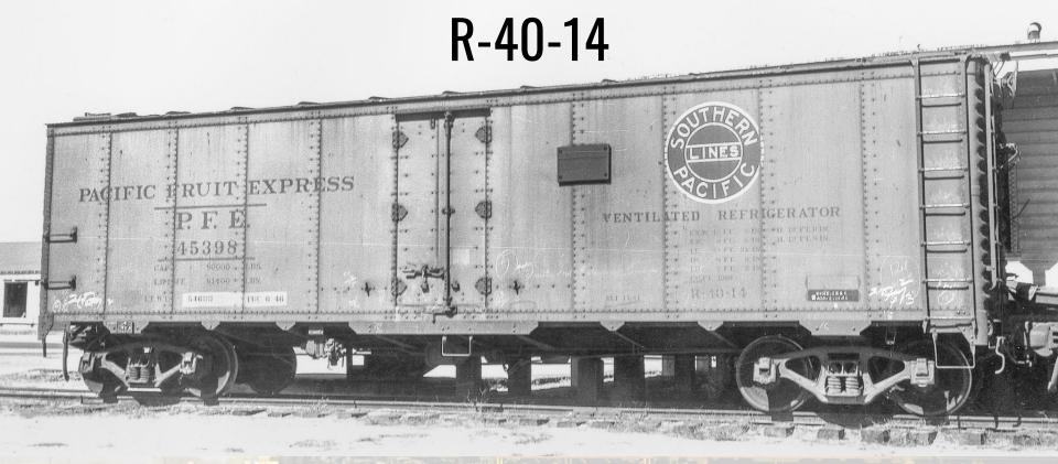
One interesting detail of dirty refrigerator cars is the stark contrast of freshly painted patches, such as the one here for the reweigh stencil
