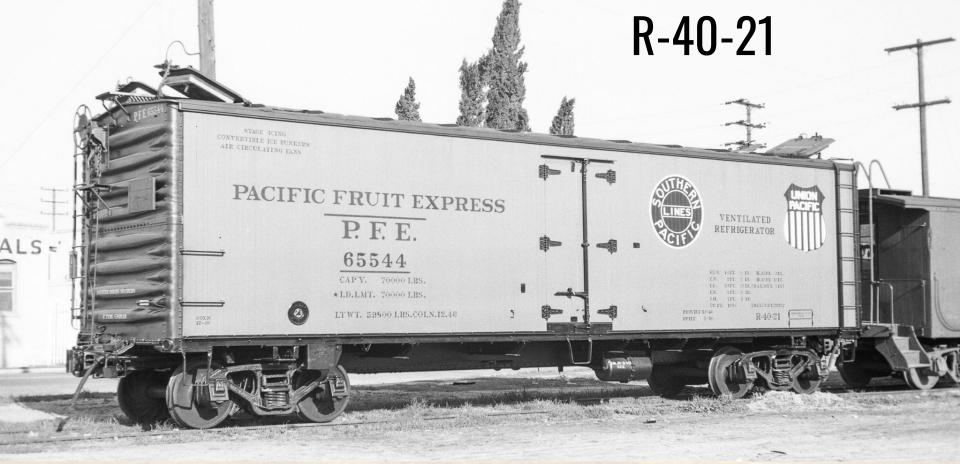
PFE 65544 was a -21 rebuild equipped with Preco FG-21 mechanical fans. Also, note the red and white stripes reversed in the UP medallion
