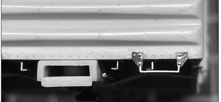
Below - the stringers and the lower right grab iron are visible in this image
