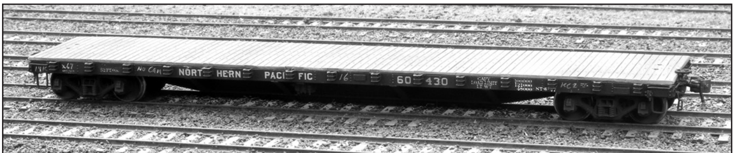
Note that the strips above the bolsters had not yet been applied in this photo.
