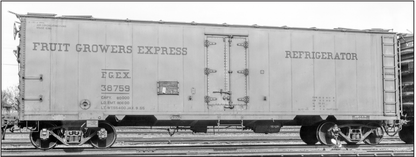
Built in July, 1948 by the Indiana Harbor shops, FGEX 38759 was part of a group of 365 cars, nos. 38635-38999, that featured welded sides, with seven panels on each side of the doors, welded underframes, long side sill supports at the car ends and under the doors, 3/3 Improved Dreadnaught ends, "Murphy" solid steel panel roofs, air circulation fans, placard boards, and wide sill steps under the doors. Courtesy of Bill Welch
