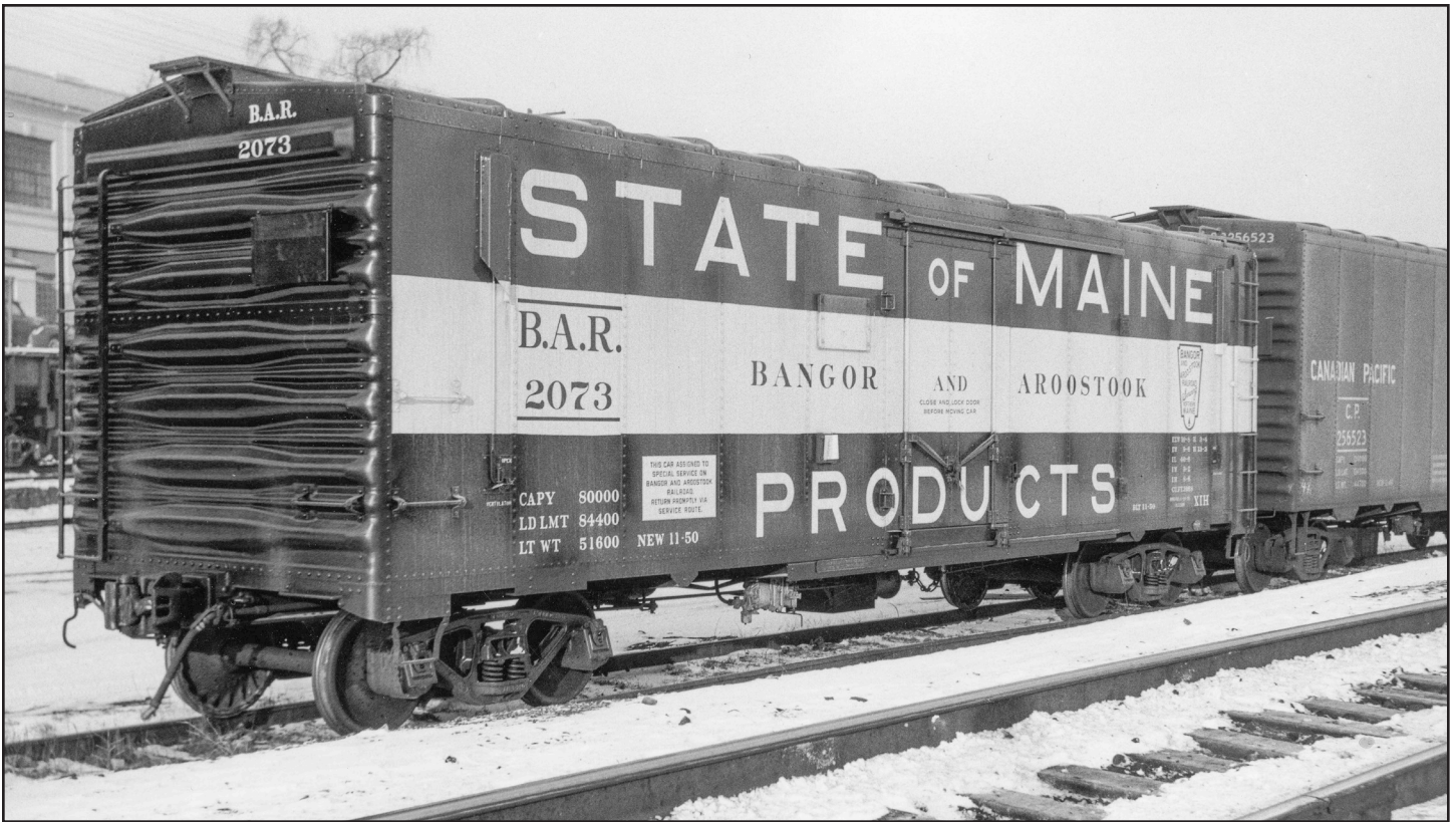
The ex-MDT cars were an expedient as BAR began to receive insulated box cars with charcoal heaters in late 1950. The cars became instantly famous for their red, white, and blue car sides emblazoned with "STATE OF MAINE" and black ends, roof, and underframe. The cars were built in two groups, the first by Magor Car Co. (car nos. 2000-2299) and used Improved Dreadnaught ends with a rectangular corrugation at top, "Murphy" solid steel diagonal panel roofs, Youngstown flush, sliding doors, and ASF A-3 Ride Control trucks. Above - Bob's Photo, below - Providence, Rhode Island, November, 11, 1957, Col. Chet McCoid photo, Bob's Photo
