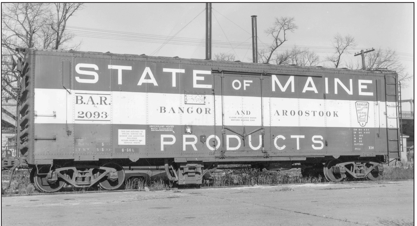
The ex-MDT cars were an expedient as BAR began to receive insulated box cars with charcoal heaters in late 1950. The cars became instantly famous for their red, white, and blue car sides emblazoned with "STATE OF MAINE" and black ends, roof, and underframe. The cars were built in two groups, the first by Magor Car Co. (car nos. 2000-2299) and used Improved Dreadnaught ends with a rectangular corrugation at top, "Murphy" solid steel diagonal panel roofs, Youngstown flush, sliding doors, and ASF A-3 Ride Control trucks. Above - Bob's Photo, below - Providence, Rhode Island, November, 11, 1957, Col. Chet McCoid photo, Bob's Photo
