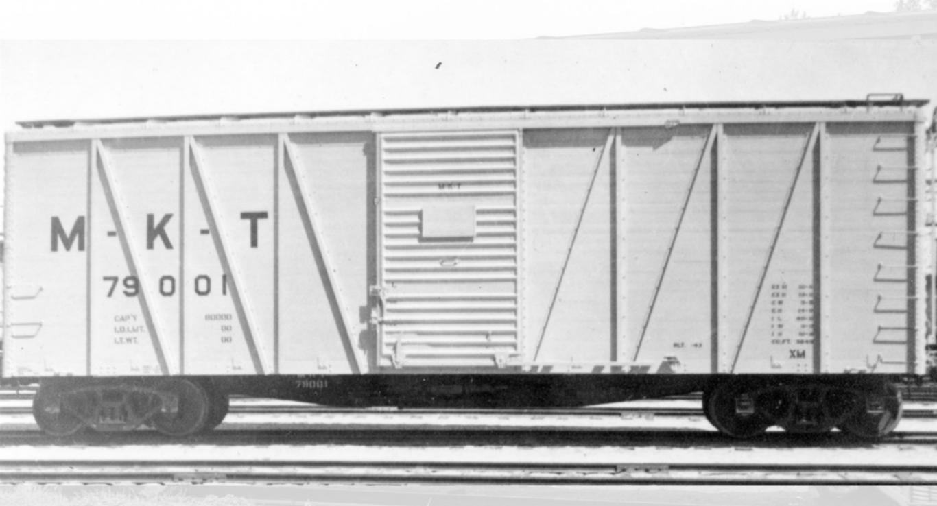
• Rebuilt at the Denison shops in 1943 from refrigerator cars (series 52001-52200, built 1923 GACC)
