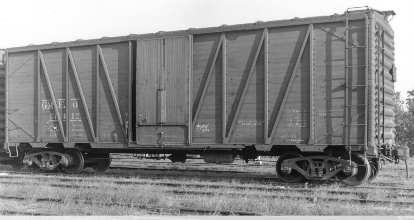
Note the Superior composite door and "repair" across the center of the door
