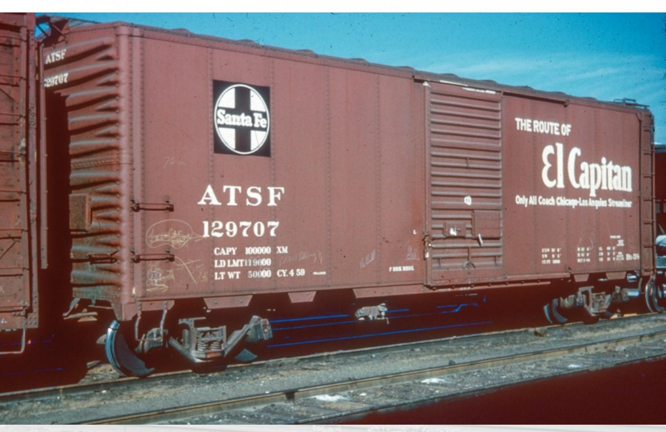
Rebuilt in 1957 with steel sides and doors
