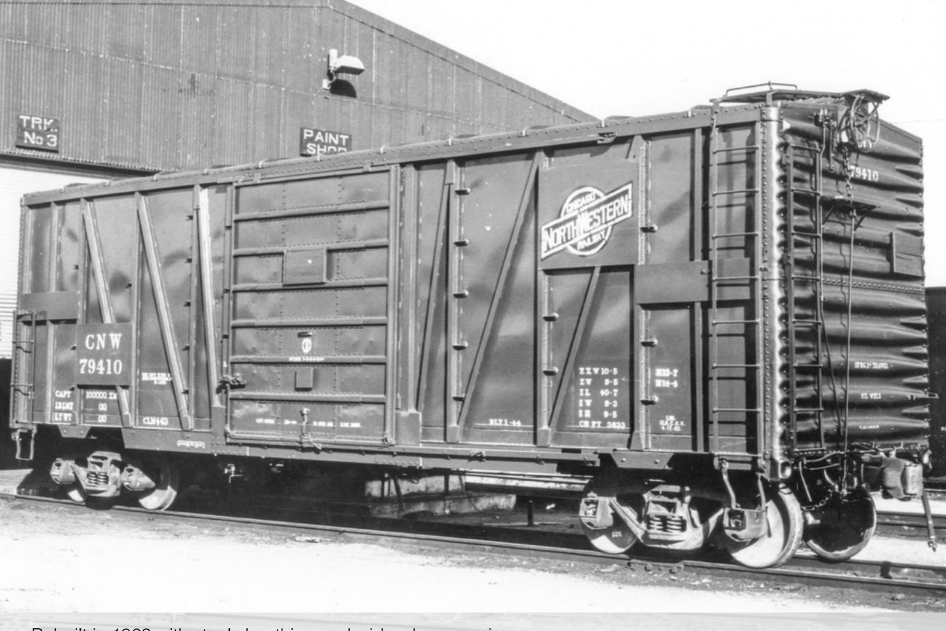
Rebuilt in 1963 with steel sheathing and wider door openings
