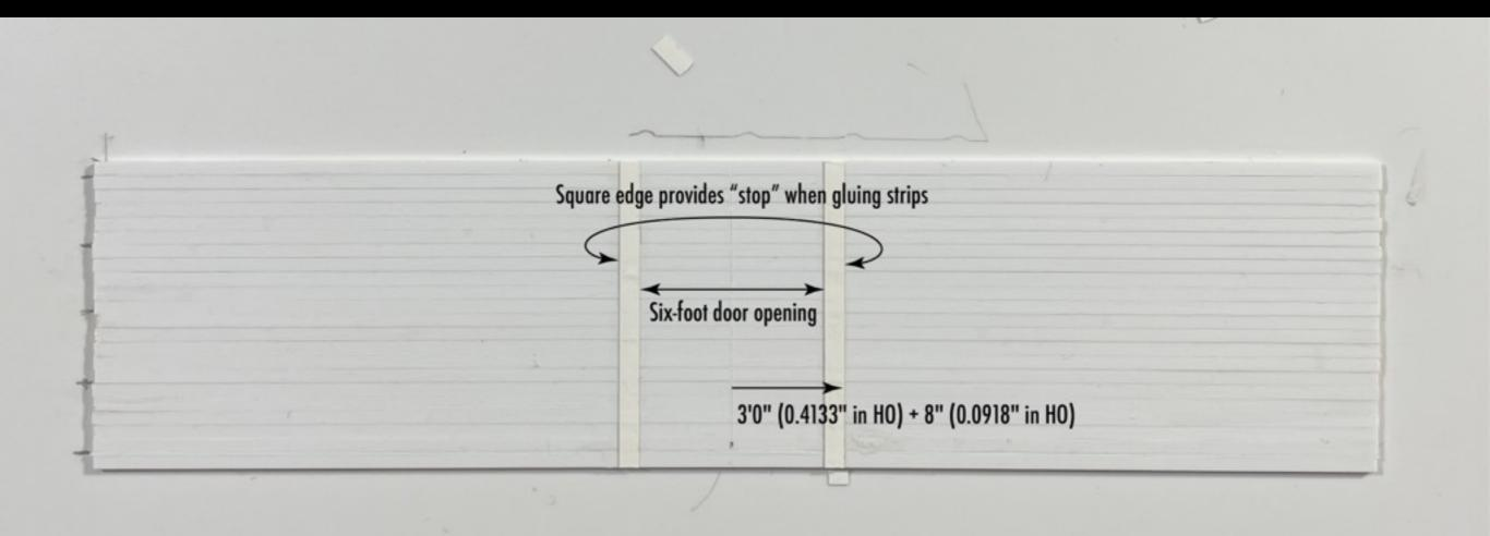
Use the edge of the square to provide a "stop"; the edge of the square is set using the calipers, set to the correct distance from the center line of the car (0.5051" in this photo)
