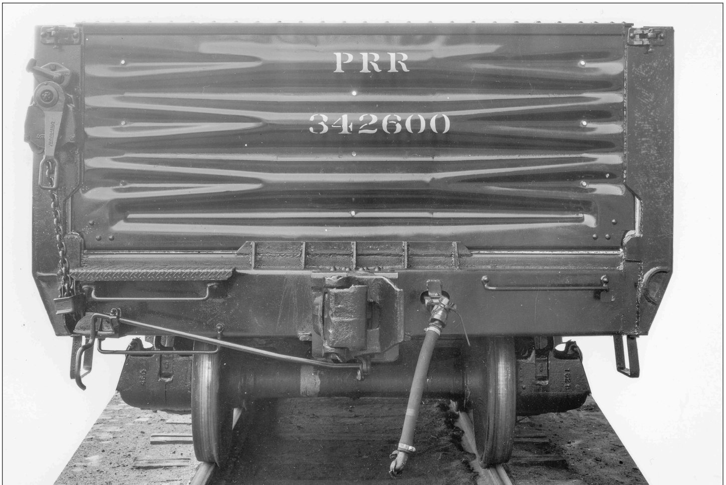
These three builder's images show many of the details of the G28 class, including two sizes of side structural members, tall(ish) sides, Dreadnaught drop ends, Universal power hand brake, National Malleable Type B 70-ton trucks, as well as the trademark Pennsy scheme with circle keystone emblem. Hagley Museum and Library
