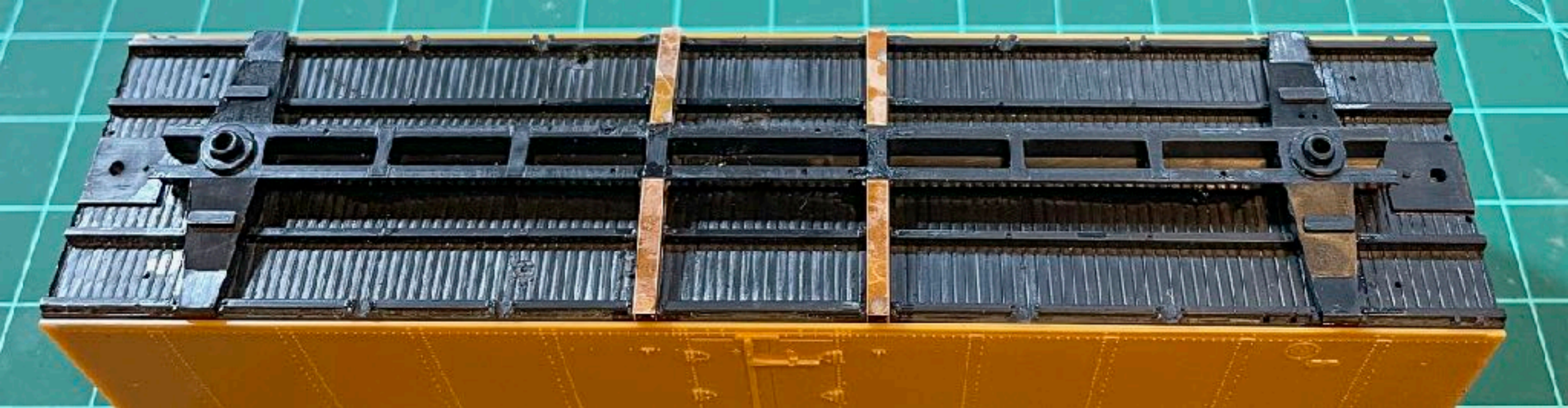
New etched and "open" crossbearers installed
